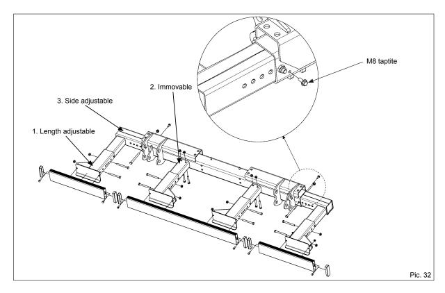
Mount each length adjustable bracket with two bolts M10x100 (8.8), each immovable bracket with two bolts M10x70 (8.8) and each side adjustable bracket with two different bolts one M12x120 and one M8 taptite (8.8) see pic. above. The taptite M8 bolt is used in order to freeze the side adjustable brackets. Tighten M10 bolts to 37 ft lbs, M12 bolts to 50 ft lbs and taptite M8 15 ft lbs
