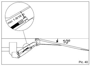
Note! The platform must not be tilted down more than max 10° below the horizontal.
