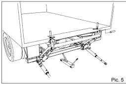
Position the support frame as required under the truck's chassis frame. eg. A wheeled jack can be used.
