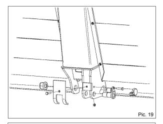
NOTE! To get the full opening speed a tilt angle sensor should be installed according to the pictures. Note! It's is important that the cable is turned in the right direction according to pictures.
