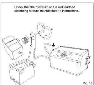
A 160 A (24 V) or 250 A (12 V) fuse is to be installed on the main power cable running from the battery compartment. Note! When passing through holes the cables must be protected with rubber bushings.
