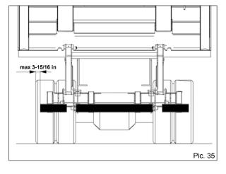
If the tail lift is equipped with auto tilt must an angle switch be installed at the lift arm.
