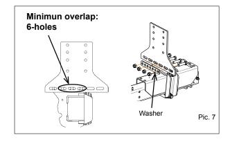
The smaller bracket can be assembled in different ways depending on the width of the truck frame. The place along the truck frame where the bracket shall be assembled is the **trucks frame width.**
