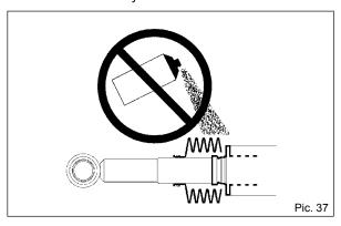
Hydraulic hoses or cables must not be painted, the paint's solvent can damage the hose's/cables rubber compound and can adversely affect durability
