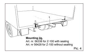
For trucks with mounting brackets kits, see separate installation instructions. See list, section 3.
