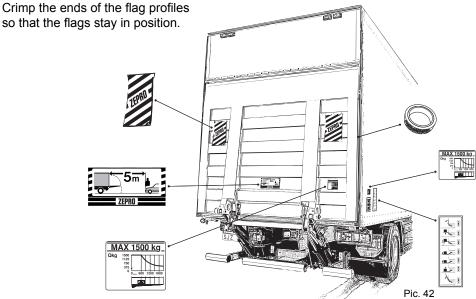
A "danger area" decal is also to be placed on the platform warning drivers who are parking cars behind the vehicle that 5m are necessary to allow for platform opening and sufficient manoeuvring space for loading and unloading goods.
