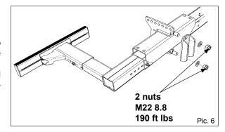
Preliminarily position the smaller bracket according to picture and fasten the two brackets to each other with screws. Use the washer between bracket and nuts. Check that there is a minimum of 6 holes overlap of the smaller bracket's row of holes.
