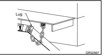
Check proper operation of lockout device.
