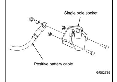
Ground trailer socket to main structure of trailer.
