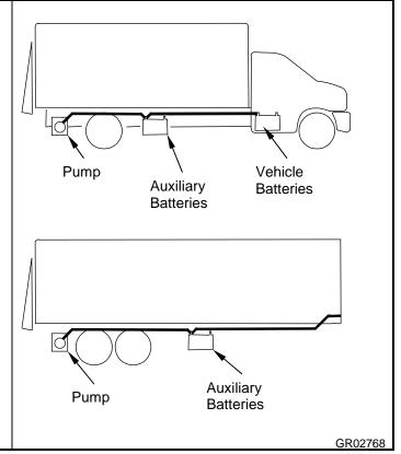
Locate battery box in a suitable location under the vehicle body.
