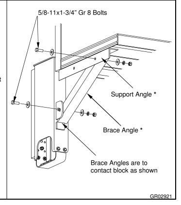
After installation of dock bumpers, ground clearance needs to be considered. If dock bumper steps are too low, they may hit the ground when driving in or out of driveways, etc.
