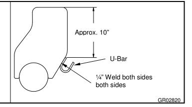
Secure wrapped hydraulic hoses in U-Bar and then hammer U-Bar closed.
