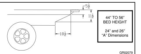
Cap Vehicle Frame, using a 3/16" or 1/4" X 2" steel strap.
