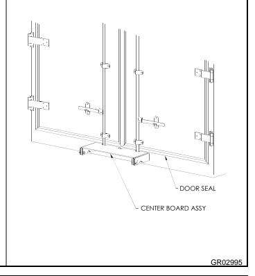
Notch Center Board to clear door locking rods and hardware.
