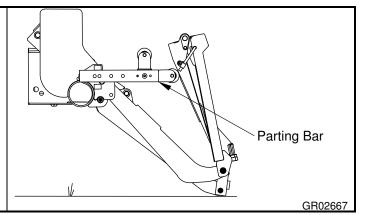
Install parting bar using #1 or #2 hole on mount tube, and A, B, C, or D hole in parting bar as indicated.
