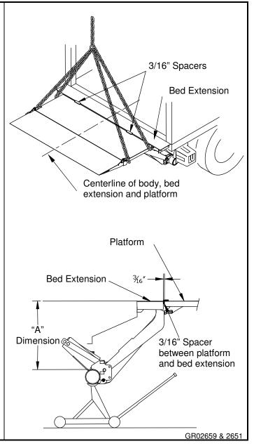
Bolts heads should be contacting platform hinges, if they are not, it may be necessary to rotate the cylinder tower towards the front of the vehicle.
