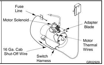
Run green 16 ga. x 40 ft. cab shut-off wire to cab shut-off switch.
