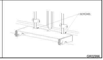
Weld Center Board to rear sill of body as shown.
