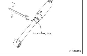
Tighten lock screws and measure the exposed cylinder threads; not to exceed more the 1-3/16"
