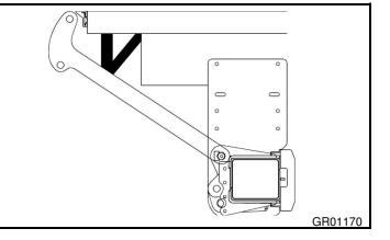
Make sure that up stops will contact lift arms as shown on drawing.
