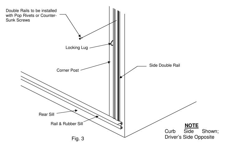
5. Insert the Rubber Seal & Air Foil down into Side Double Rails from the top as shown.
