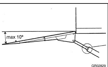
Loosen the cylinder ring's lock screw (1). Screw the ring out in the direction of the platform (2)
