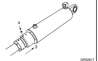
Reassemble the rubber bellows as shown to the following A dimensions:
