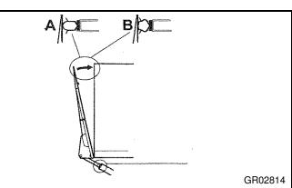
Loosen rubber bellows and loosen (3) lock screws.
