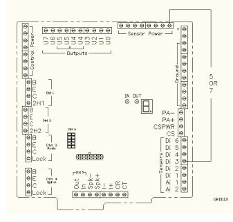
For units without an inside of deck mounted angle sensor, verify there is a Green or Red jumper wire installed between "Sensor Power" and Di 3 terminals on circuit board.
