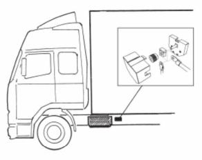
NB. The quick connectors must be well protected and should be positioned inside the vehicle chassis.
