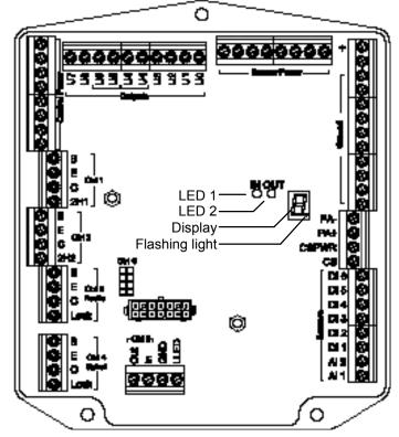
Image 2. The control card is equipped with an alphanumerical display with a flashing light and 2 red LEDS
