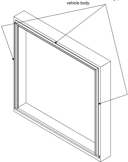
Add silicone caulk to seal gaps between tracks and vehicle body.
