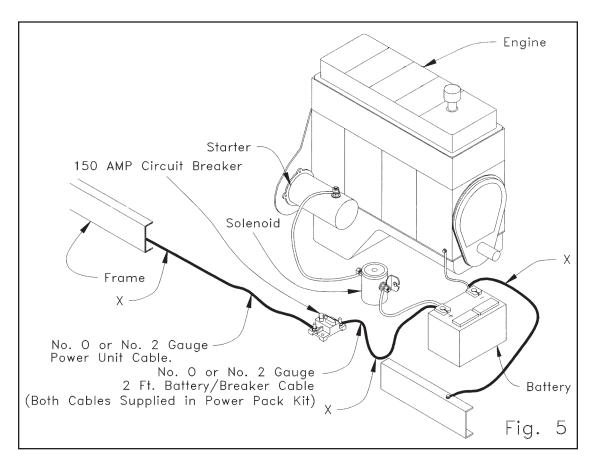
Step 7 Many late model trucks have battery connections as shown in Figure 5. The ground cable from the battery is connected directly to the engine block with only a light braided ground strap from the block to the chassis (either the body or the frame.) Where this is the case, the factory-installed wiring usually does not provide an adequate ground circuit for battery-operated accessories, such as electric-hydraulic tailgates.
