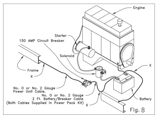
**Step 15** Many late model trucks have battery connections as shown in Figure 8. The ground cable from the battery is connected directly to the engine block with only a light braided ground strap from the block to the chassis (either the body or the frame). Where this is the case, the factory-installed wiring usually does not provide an adequate ground circuit for battery-operated accessories, such as electric-hydraulic tailgates.
