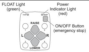
Turn the vehicle ignition switch to the "ON" or "ACCESSORY" position. The control backlight will illuminate.  Press the ON/OFF button on the control. The power indicator light glows red, indicating that the control is ON. The indicator light glows red whenever the control and the vehicle ignition switch are both ON, the electrical connections to the snowplow are completed, and the plow power switch is in the "PLOWING" position.
