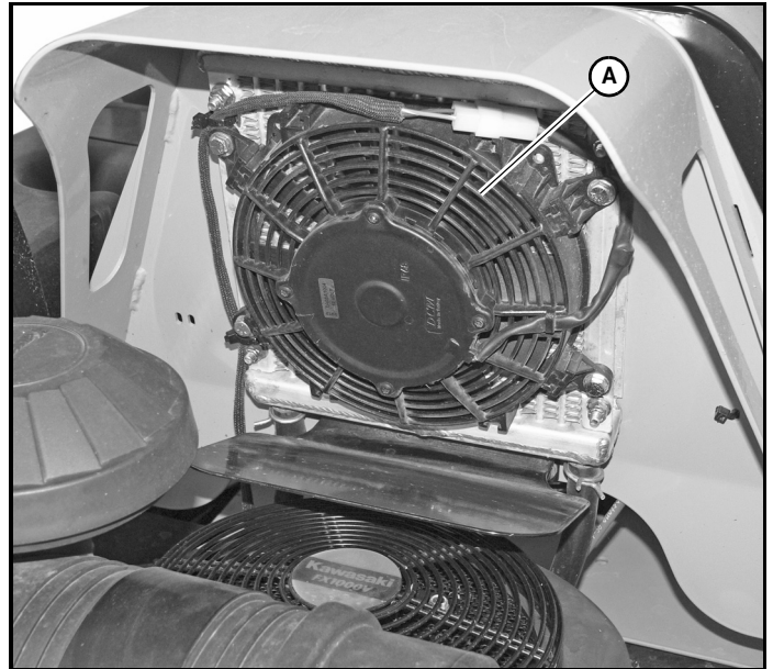
A. Heat exchanger
