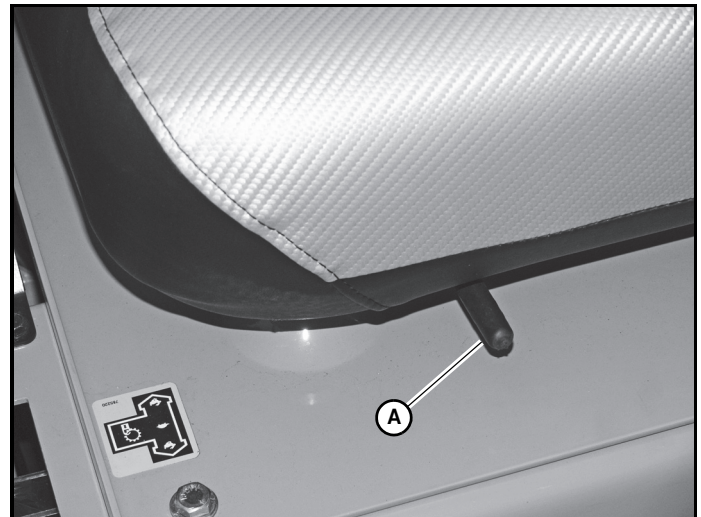
A. Seat release lever
