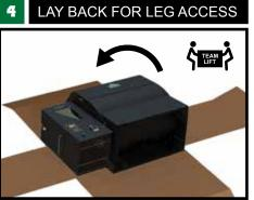
Lay grill down on it's back. Keep on cardboard to prevent scratches.
