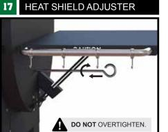
Insert adjuster handle into hole on right side of grill wall and screw into head shield.
