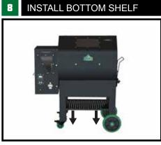
Slide shelf down to sit on shelf arm bolts. Align with grooves under shelf.
